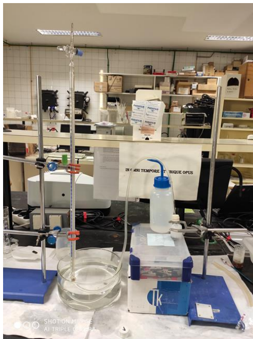
Figure S2. Set up for hydrogen production measurements
