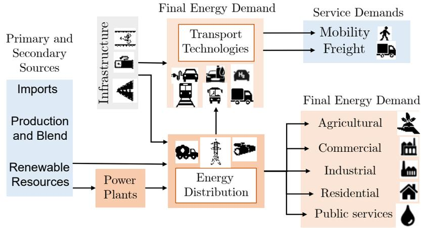
**Figure 2.2:** Reference Energy System (RES) of OSEMOSSYS-CR.
