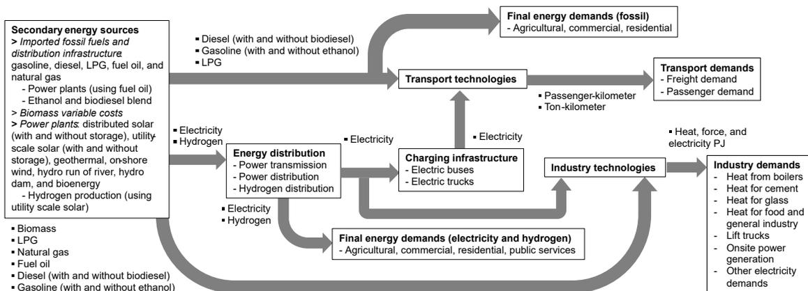
**Figure 3.3:** Reference energy system for the energy, transport, and industry sectors. Based on Victor-Gallardo, Rodríguez-Zúñiga, Rodríguez-Arce, et al., 2022.
