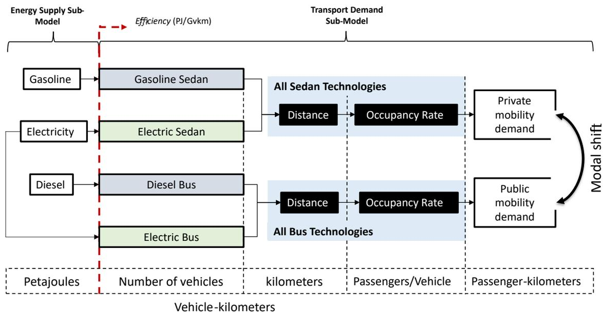
**Figure 2.5:** Transport modeling in OSeMOSYS-CR.
