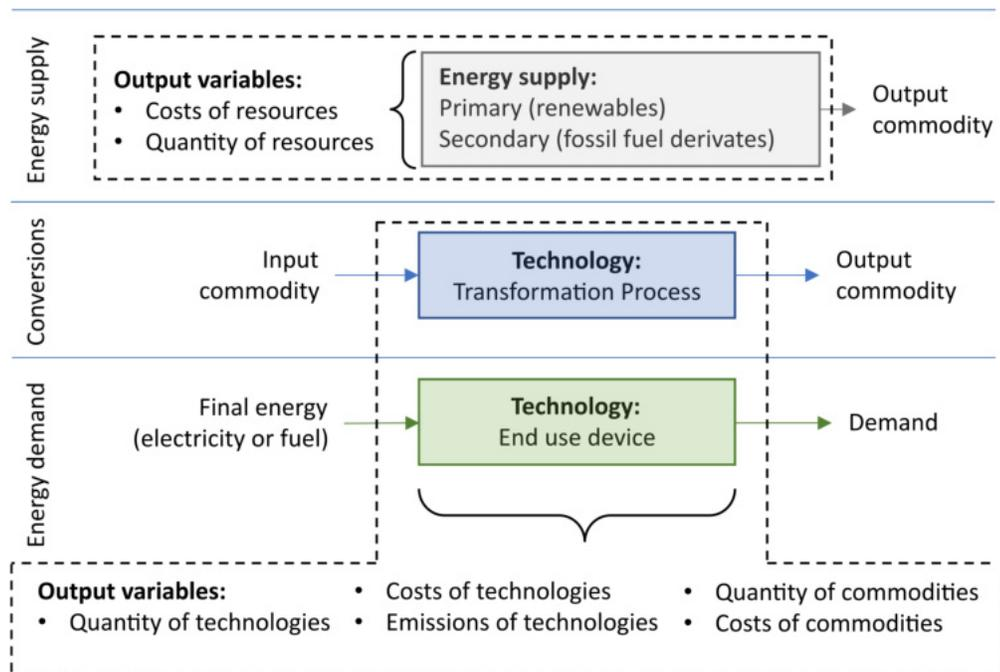
**Figure 2.3:** Outputs of RES elements.
