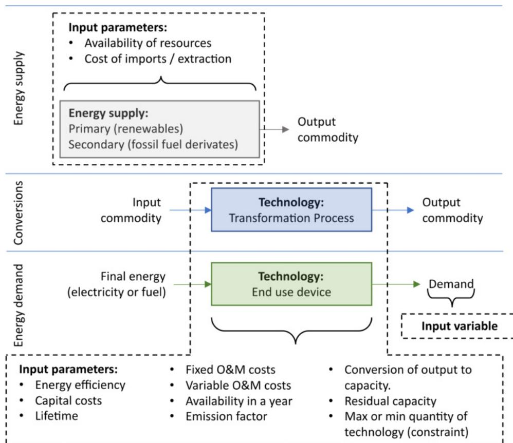
Figure 2.4: Inputs of RES elements.
