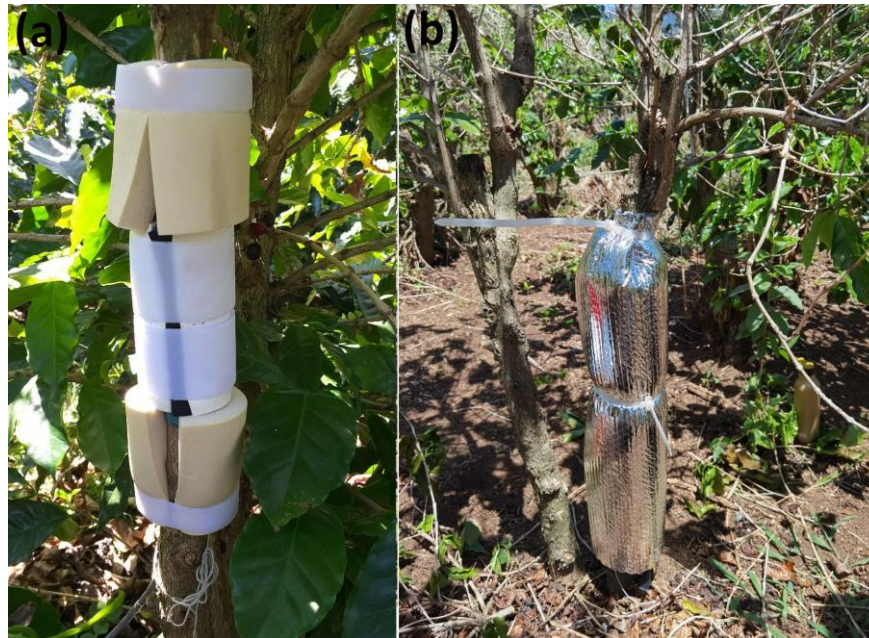
Figure 2.3 (a) Installation of the sap sensor in coffee. (b) Sap sensor once installed and collecting data at La Hilda.
