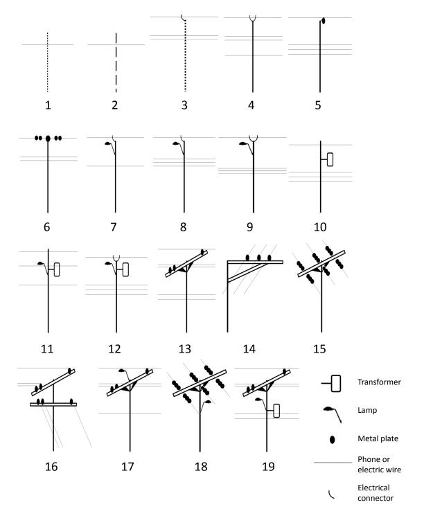
Figure 1. Scheme of electric pole types. Continuous black lines represent poles made of concrete, the dotted line poles made of wood, and the dashed line poles made of metal.
