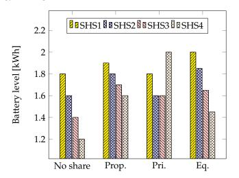
**Figure 7.** Battery energy levels for the 4 SHS batteries without sharing and after the combined excess energy distribution based on proportional (Prop.) energy sharing, priority (Pri.) energy sharing, and equal (Eq.) energy sharing. The rated battery capacity is also shown as the dashed line in the plot.
