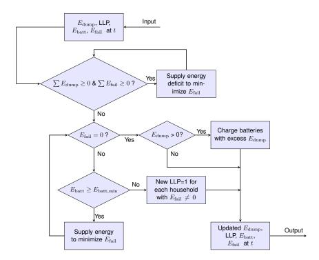
**Figure 6.** Algorithm for sharing the excess energy based on the ranking of load deficit (in terms of  $E_{\text{fail}}$  and battery depth of discharge (DOD)).
