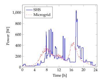
**Figure 8.** Comparison of 1-day load profile for a tier 4 standalone SHS and an average load profile for the SHS-based microgrid with 50 households for the same day. The demand diversity can be seen to significantly reduce the peak average load.
