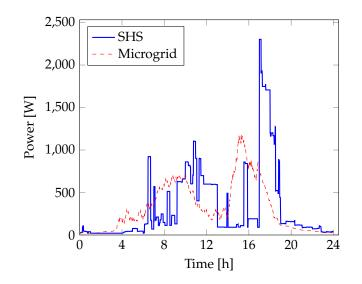
**Figure 9.** Comparison of 1-day load profile for a tier 5 standalone SHS and an average load profile for the SHS-based microgrid with 50 households for the same day. The demand diversity can be seen to significantly reduce the peak average load.
