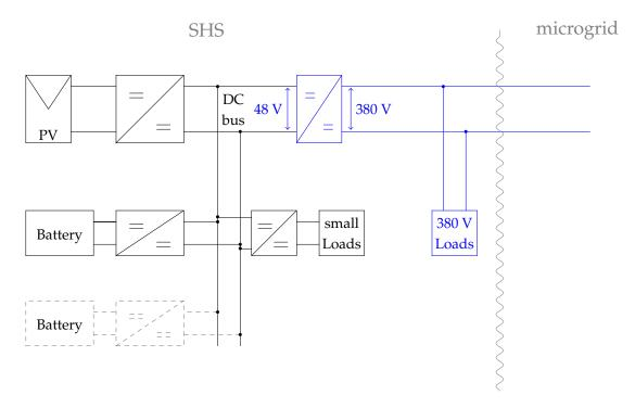
**Figure 3.** Modular DC architecture for an SHS-based DC microgrid that enables intra-household growth option as well as scalability in the form of a meshed DC microgrid. Dashed battery with converter illustrates the modular capability. Similar modular expandability can be considered for loads and PV too. The additional hardware needed to go from standalone SHSs to microgrid, along with the high power loads at 380 V that the microgrid can support, are denoted in blue colour.
