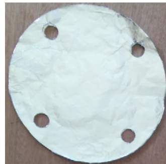
Figure 3. Shock tube prototype diaphragm.
