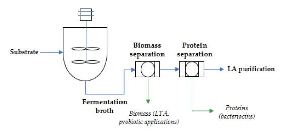
**Figure 3.** Potential process flow diagram for of a multi-product LAB based process (adapted from Reference [147] licensed under CC BY-NC 4.0 available at https://doi.org/10.1016/j.jclepro.2019.119165).
